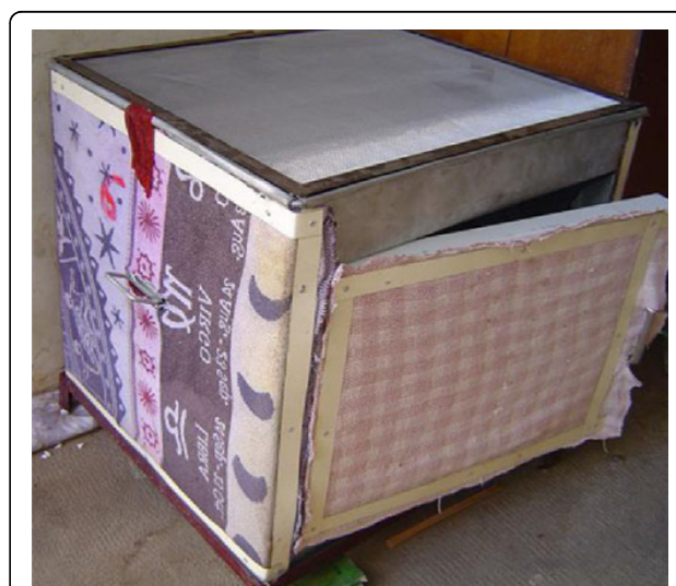
Figure 1 Photo of ‘Cambodian Cooler Box’ (CCB). A cloth wick connects the water reservoir contents to the cloth sides except on the side with the door
